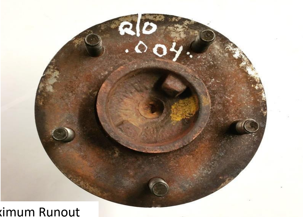
Bearing Journal out of Tolerance. 1.375" and 1.187" Minimum
